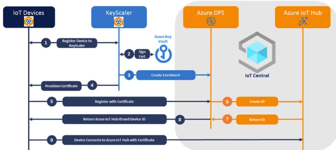
Step 1 - When a device powers up, it connects to KeyScaler and registers to the platform (assuming it is an authentic device)
